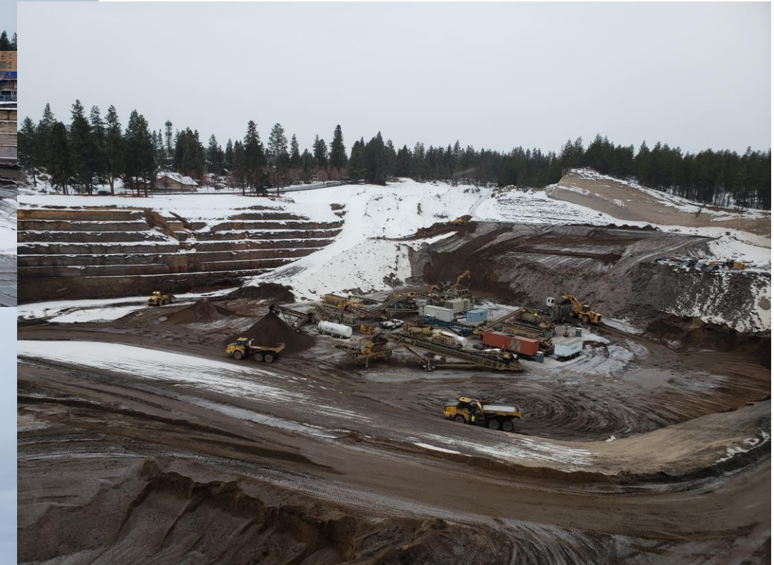
Trommel being setup for screening in Cell 1
